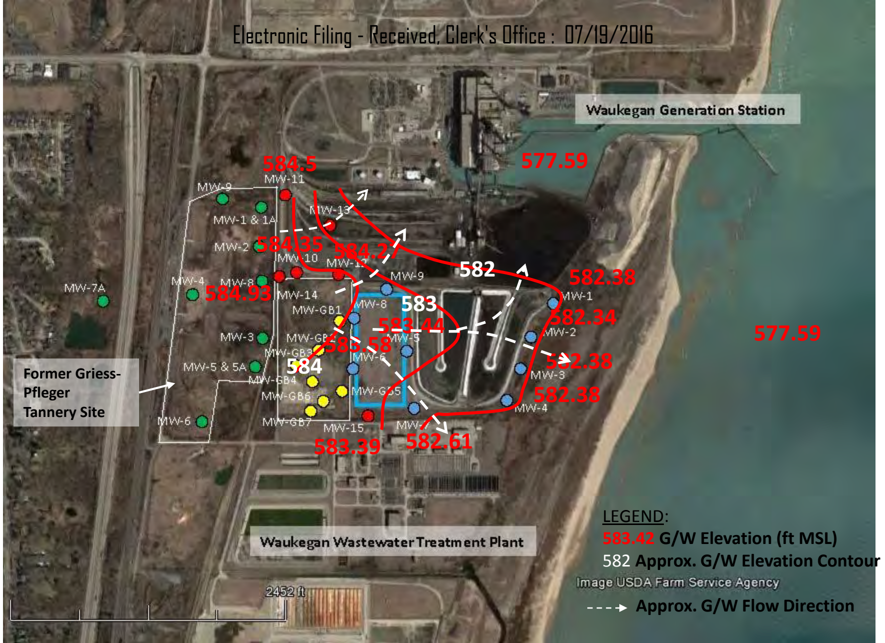
Figure 20 Approximate Ground-water Contours June 2013 (PCB 2013-015)
