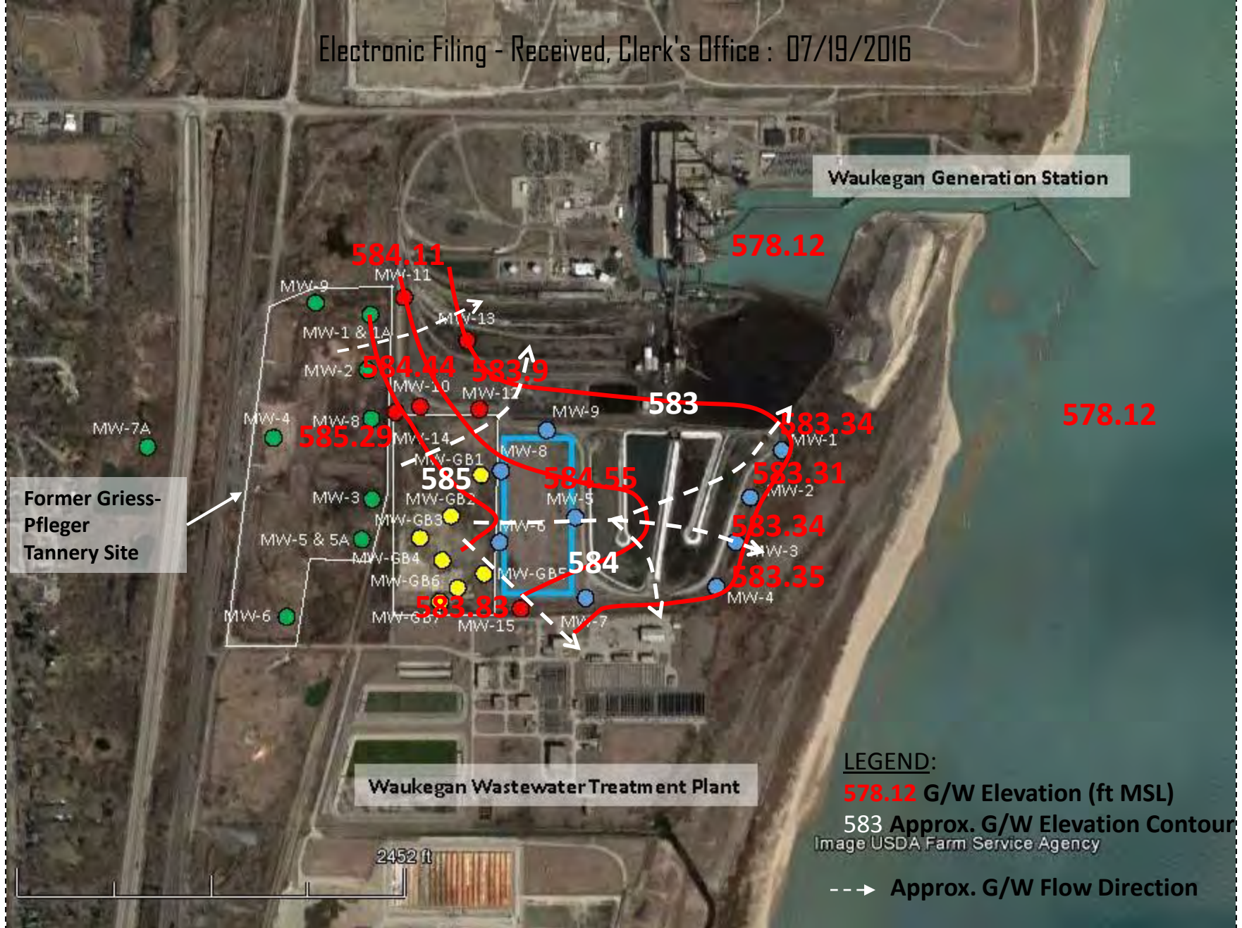
Figure 18 Approximate Ground-water Contours June 2011 (PCB 2013-015)
