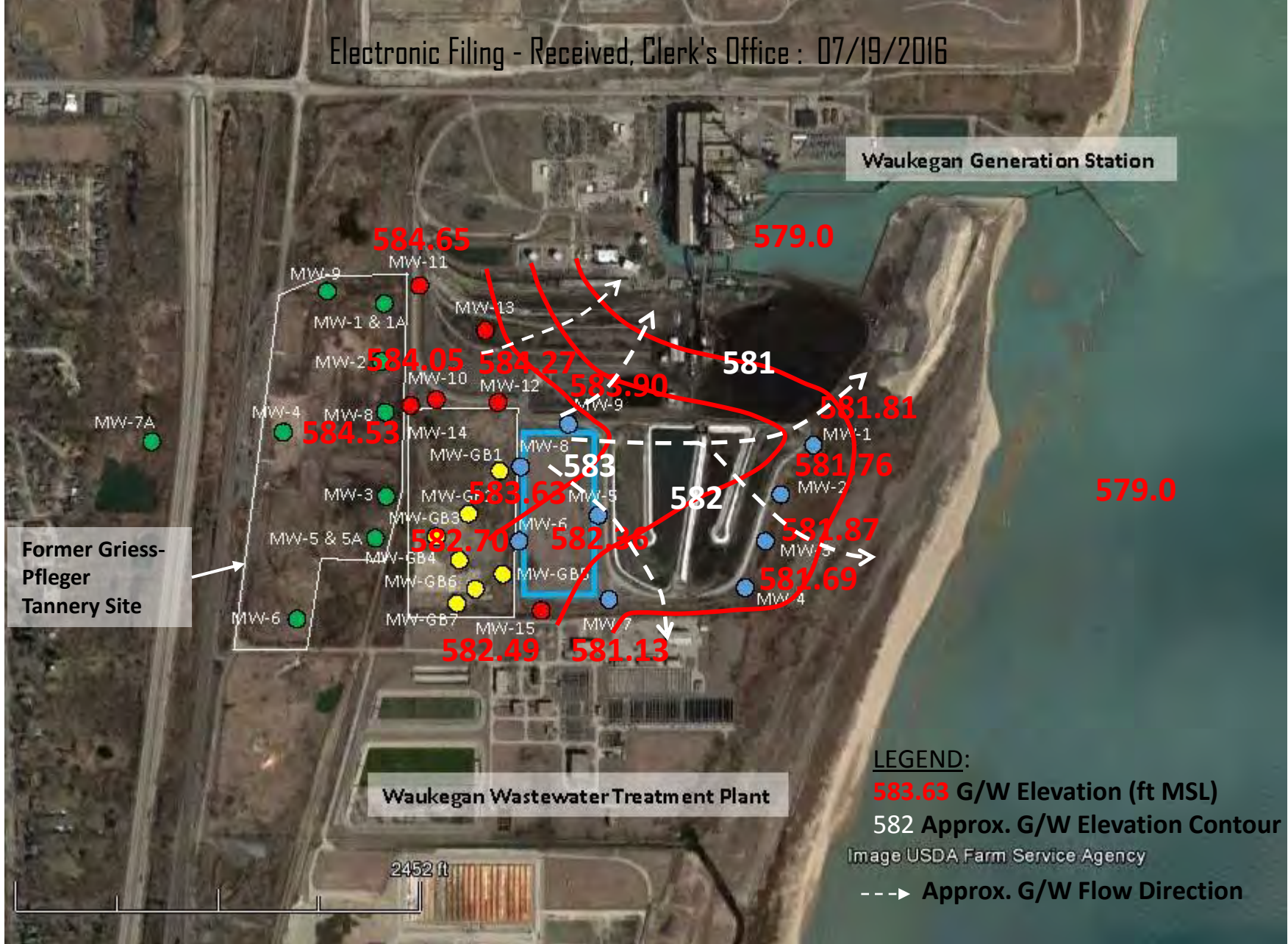
Figure 21 Approximate Ground-water Contours August 2014 (PCB 2013-015)
