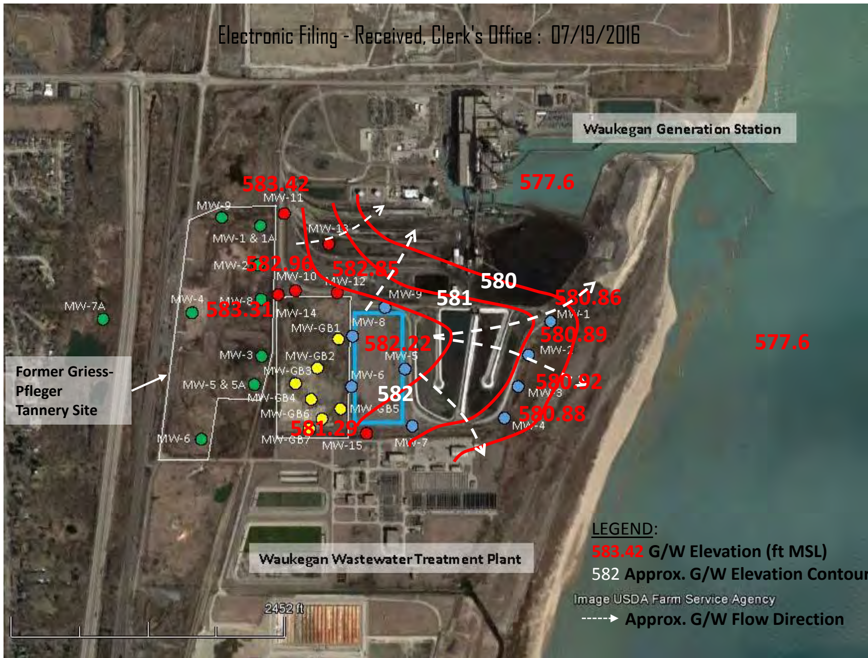
Figure 19 Approximate Ground-water Contours June 2012 (PCB 2013-015)
